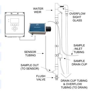
CRIUS® FilterSense with overflow weir
