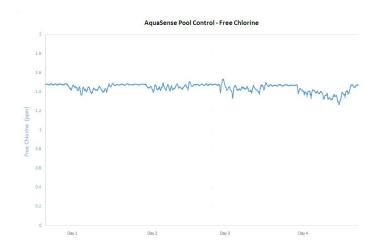
Being able to accurately measure the chlorine and respond to varying bathing loads means that pools and spas can operate at lower chlorine levels, reducing the formation of unpleasant combined chlorines and reducing the chemical usage, thereby reducing costs and reducing emissions, all while providing a better bathing experience.
